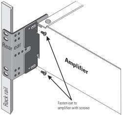
Optional rear rack mounting ear attachment methodsrefer to the rear rack mounting ear kit's documentation for details
